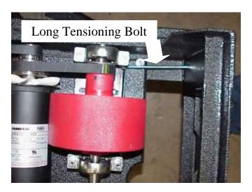
Use a ½" socket wrench to tighten the tensioning bolt just enough to remove the slipping. Check the tension on the belt that runs from the motor to the front roller by twisting or wiggling it. You should be able to twist the belt about 90 degrees.
