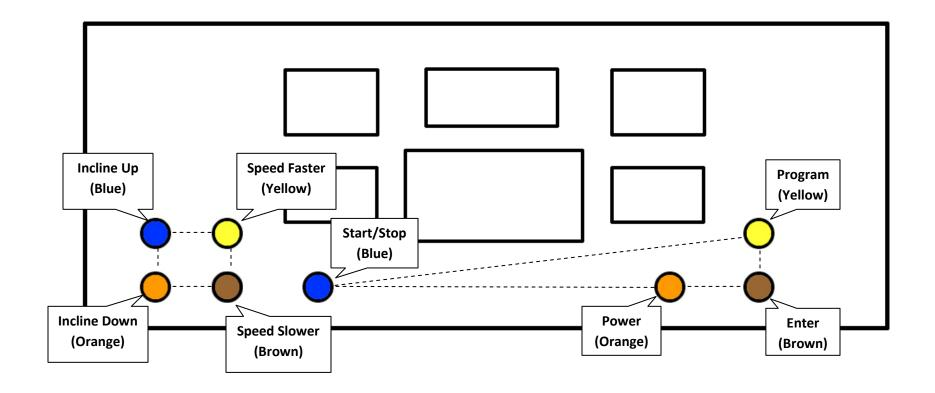
Button positions connected by a dashed line are from the same wiring harness.
