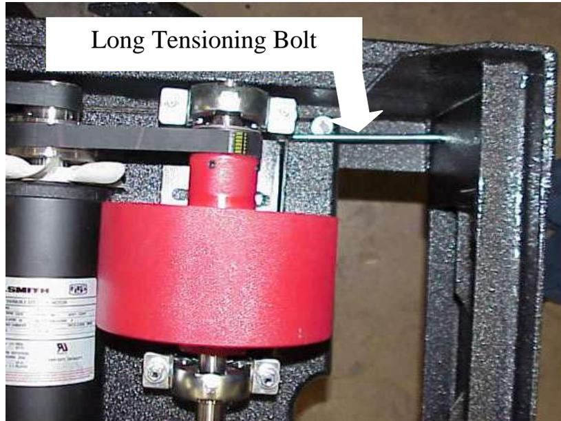
Use a ½” socket wrench to tighten the tensioning bolt just enough to remove the belt slipping.
