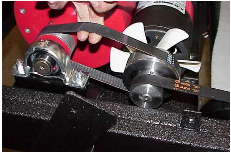
If you wiggle the belt up and down, there should be at least 1" of play. Be careful not to over-tighten the flywheel belt. **Over-tightening the flywheel belt can cause the motor shaft to snap and void the warranty.**
