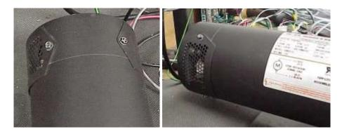
Place one of the brushes back into its slot and replace the clip that holds it in place. Repeat this step for the brush on the other side of the motor. The contour of the brush <u>must</u> match the contour of the motor, or the brush will not make proper contact with the commutator.
