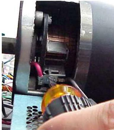
Slide the brush back in place in the top part of the slot, and hold in place while re-inserting the clip.
