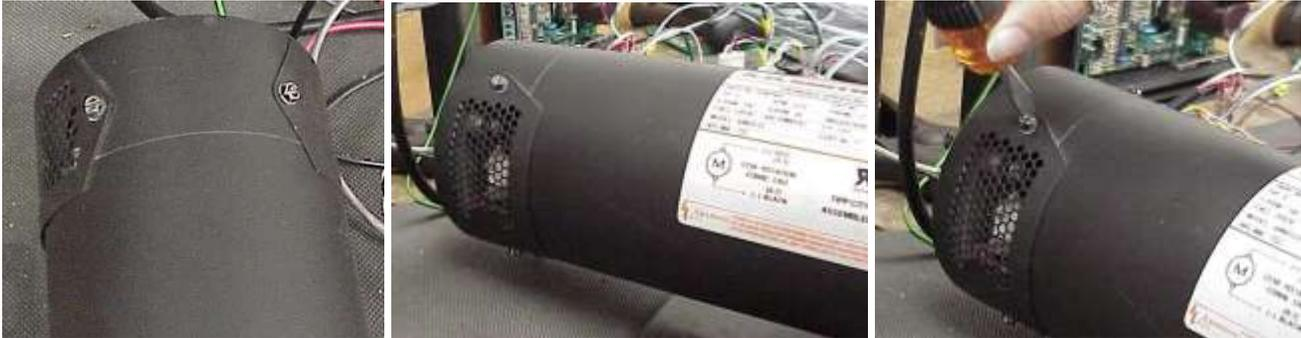
Locate the brush and the clip holding it in place. On one side of the motor, the clip will be under the brush, and on the other side it will be on top of the brush.
