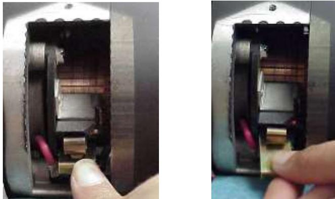
Pull the brush out of the slot and check the size. If the longest side is less than  $\frac{3}{4}$  inch long, replace both brushes in the motor.
